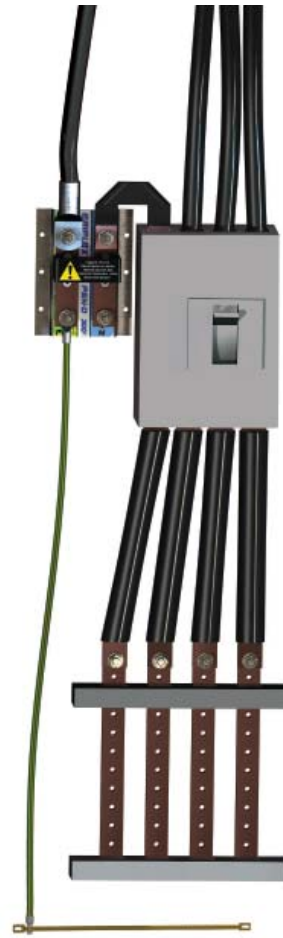
Dedicated TN-S Power Supply
